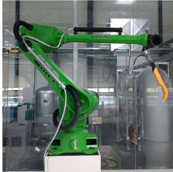
Figure 8: An industrial spray painting robot.
